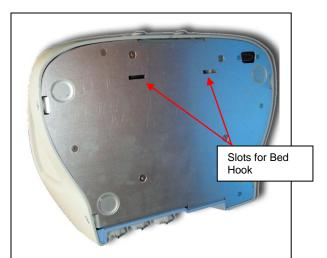
**Step 1:** Tip the unit onto its side so that the bottom panel is accessible.
