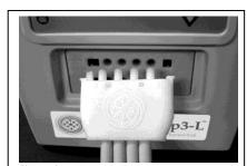
Step 4: Line up and install connector end into the unit. Squeeze the sides of the connector while pushing into the ports of the unit until flush and connector locks into place (Step 5).
